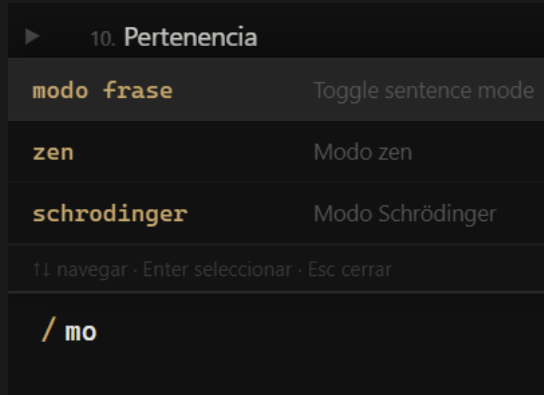
Figure 3.2 — Activating Sentence Mode from the Terminal: type / to open the command menu and choose "sentence mode", or type the command directly.
